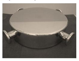
The weights will be calibrated at the beginning and end of the circuit by a laboratory accredited to ISO 17025 in order to study stability. The laboratory's expanded uncertainties (k=2) U are:
